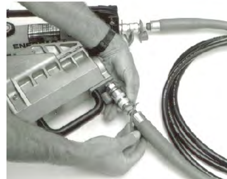
Figure 18: Installing Jaw insert and connecting tooling to pump
