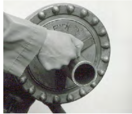
Figure 9c: Sanding Preparation Inspection
