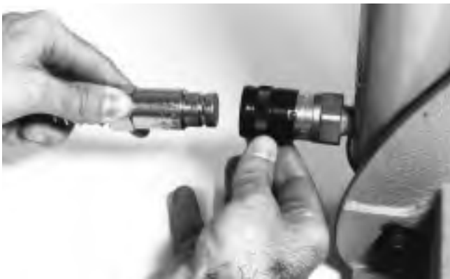
Figure 3 – Connecting Hydraulic Foot Pump to Cutter
