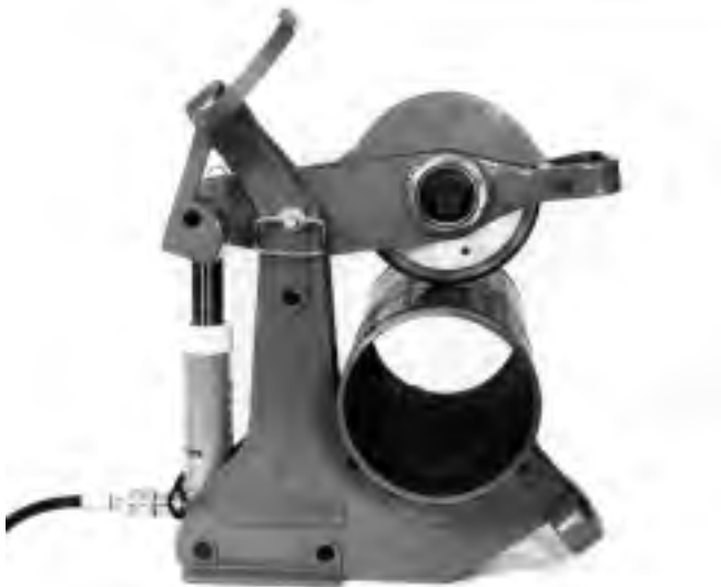
Figure 8 – Positioning Pipe in Cutter
