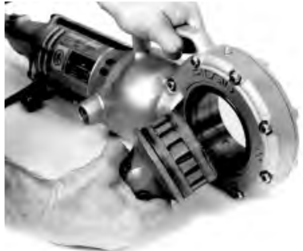
Figure 4 – Installing 774 Drive Adapter
