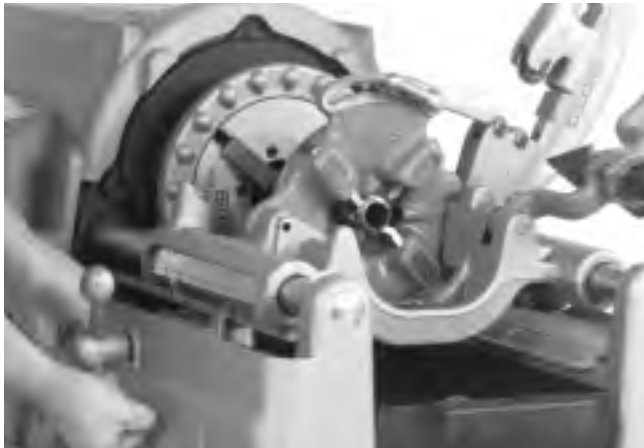
Figure 8 – Threading with 535 Manual Threading Machine
