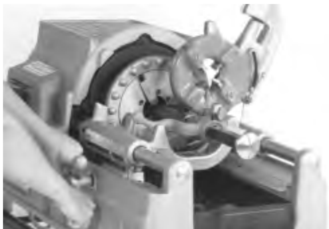
Figure 7 – Reaming with 341 Reamer
