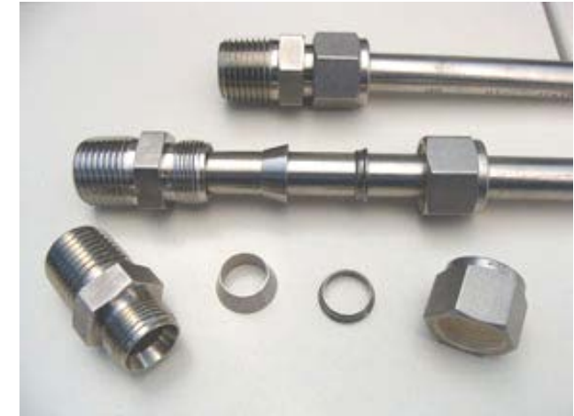
Note order and orientation of fitting components. (Body, front ferrule, back ferrule, nut)
