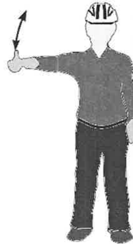
RAISE boom Signal with one hand. Right arm stretched outwards, thumb pointing upwards.
