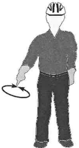
LOWER load Right arm down, palm of the hand facing inwards, moving slowly in a circle.
