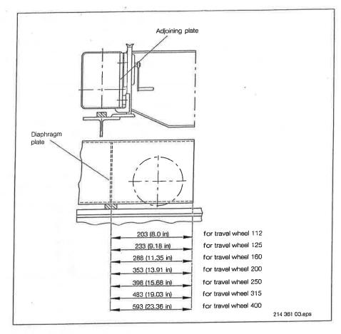
Jacking-up the endtruck is necessary for certain fitting operations so that the load is removed from the travel wheels (wheel block).
