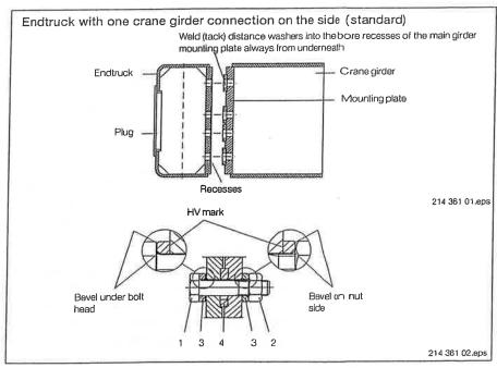
The recesses on the endtruck and the distance washers on the mounting surfaces of the connecting sleeves and the bore holes in the girder mounting plates must be free from rust, dust, grease, paint and other contaminants.
