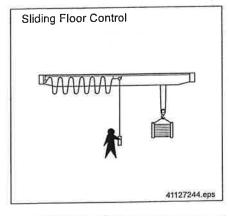
The sliding floor-level control pendant can travel along the crane girder and is located independently of the trolley. It allows the operator to move freely, to avoid obstacles and to maintain safety distances at an optimum position in relation to the load. This type of control is permitted for travel speeds up to 175 ft/min.
