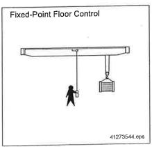
The fixed-point floor control system is used where the operating or travel path runs parallel to the crane runway. In this case direct load guidance by the operator is not always possible.
