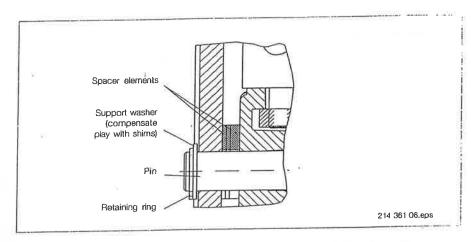
Adjusting the span Demag DRS wheel block system By re-arranging the spacer elements, the span can be adjusted. The standard as-signment and the max. adjustment possibilities are specified in the following table.
