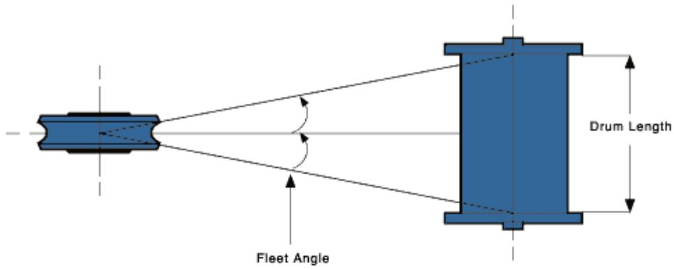
**Minimum Distance from Drum to First Sheave or Load Connection - Feet**
