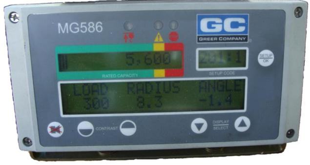
Microguard 586 Rated Capacity Indicator/Limiter System is a visual and audible alert system used in the operation of industrial cranes.
