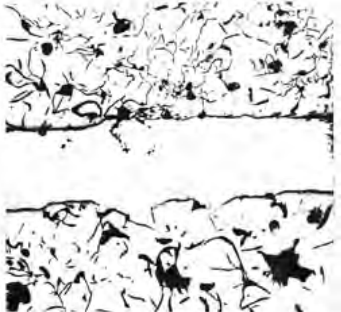
Fig. 2 Argon-braze 49H fills a surface crack on high phosphorous grey iron.
