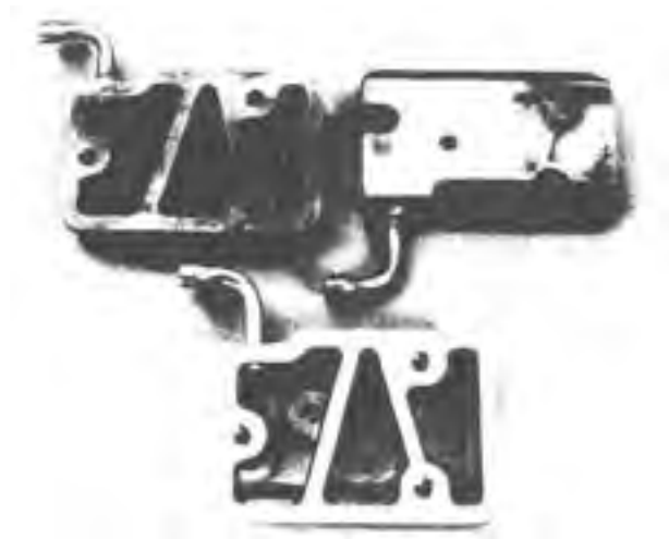
Fig. 3 Grey iron compressor discharge muffler cover brazed to steel tubing. Joint is fully penetrated.
