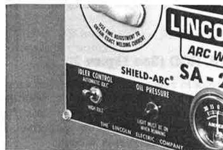
Figure 5 — Idler Control Switch.
